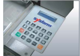
▲ 20 programs with 9 steps each Fully programmable backgauge 10 push button key pad and memory for repeat cuts
